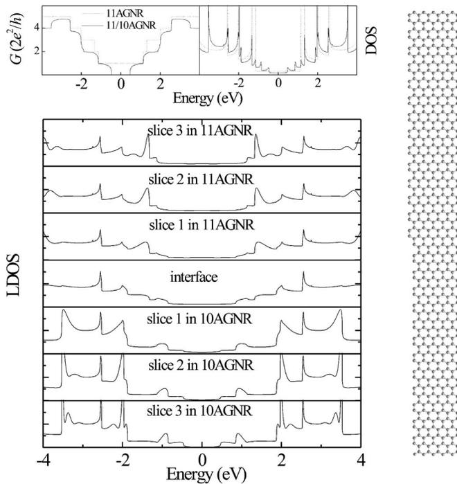
FIG. 1. 11AGNR/10AGNR metal/semiconducting junction: (Top) Conductance and DOS of the whole system. (Bottom) LDOS at slices near the interface. Slice  $n$  ( $n=1, 2$ , and  $3$ ) represents the  $n$ th nearest slice to the interface and the vertical scale of DOS is  $0.2$ .
