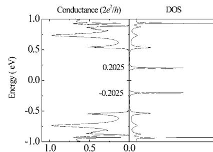
FIG. 3. Quantum dot structure based on 12AGNR/11AGNR/12AGNR junction: (Top) Conductance and DOS at low bias, where two isolated sharp peaks appear inside the gap. (Bottom) Spatial-resolved LDOS at  $E=0.2025 \text{ eV}$ ; the gray dot represents the ionic site and the radius of the circle around it corresponds to the value of LDOS.
