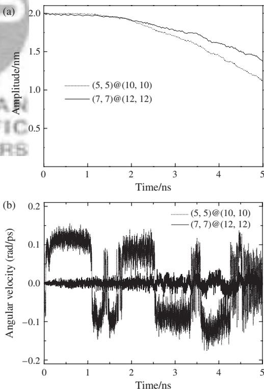
**Fig. 4.** Effects of the angular potential barriers on the energy dissipation of sliding. (a) Oscillatory amplitude damping of (5, 5)@(10, 10) (dot) and (7, 7)@(12, 12) (solid line) nanotubes, (b) corresponding angular velocities excited during the axial sliding.
