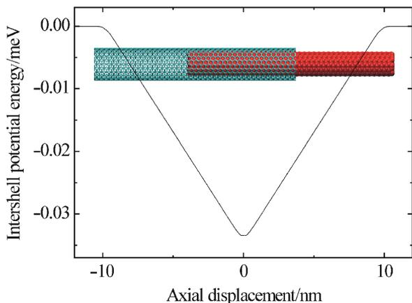
**Fig. 1.** The atomic configuration of the double-walled carbon nanotube (5, 5)@(10, 10) based mechanical oscillator and the potential profile along the axial displacement between the centers of the mass in the inner (red) and outer tube (gray) respectively.
