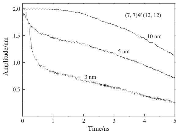
**Fig. 5.** Decaying of the axial oscillatory amplitude in the double-walled carbon nanotube (7, 7)@(12, 12), with different length of 3 (dot), 5 (dash-dot) and 10 nm (solid line) respectively.
