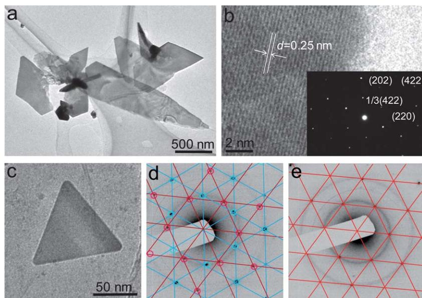
**Fig. 4** TEM images and SAED patterns of Ag nanoplates. (a–c) TEM images. The inset of (b) shows the SAED pattern with plane index. (d) Superimposed SAED pattern with blue grids for Ag *fcc* lattice and red grids for graphene hexagonal lattice. (e) SAED pattern taken at a nearby location from sole graphene for identification of the graphene lattice in the superimposed pattern.
