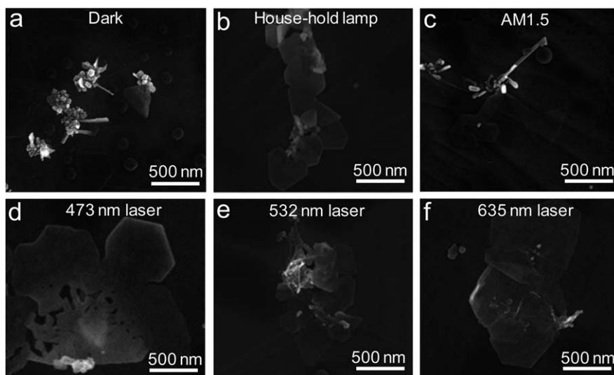
**Fig. 3** SEM images of light-induced Ag nanoplates obtained under (a) dark, (b) faint fluorescent light, (c) simulated solar light (AM1.5), (d) 473 nm blue laser, (e) 532 nm green laser, (f) 635 nm red laser.
