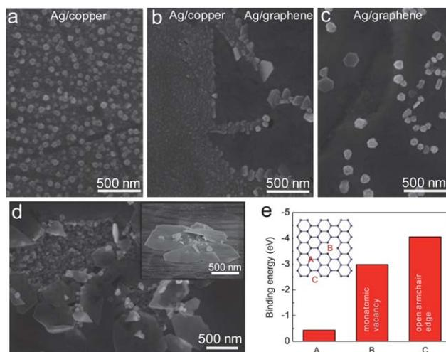
**Fig. 2** SEM images of Ag nanostructures. (a) Nanoparticles deposited on bare copper surface. (b) Morphology transition near the boundary between copper (left) and graphene (right). (c) Nanoplates deposited on graphene. (d) Nanoplates grown over cracks on graphene. Inset: tilt-view of nanoplates on graphene. (e) Binding sites and energies of an Ag atom on a graphene sheet. A: on the top of the basal plane, B: on the top of a monatomic vacancy, C: at the armchair edge.
