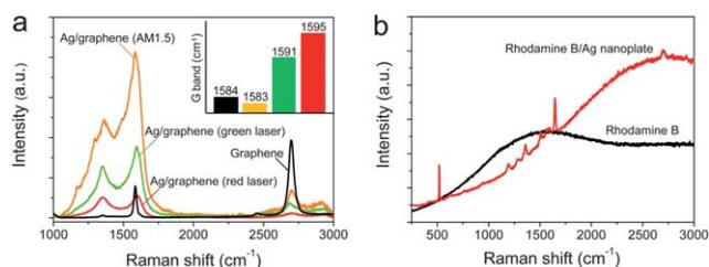
Fig. 5 (a) The Raman spectra of light-induced graphene–Ag hybrids. (b) SERS of Rhodamine B.
