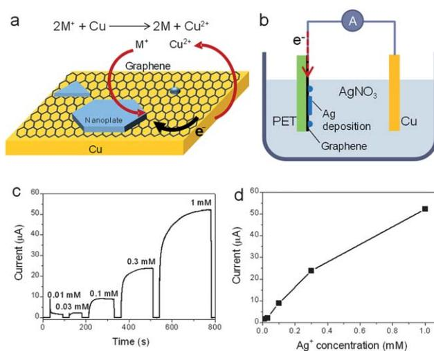
**Fig. 1** (a) A schematic of *in situ* galvanic synthesis of graphene-Ag hybrids. (b) Schematic of a primary battery made from graphene/PET and copper. (c) Output current of the primary battery. (d) Correlation between the output current and  $\text{Ag}^+$  concentration.
