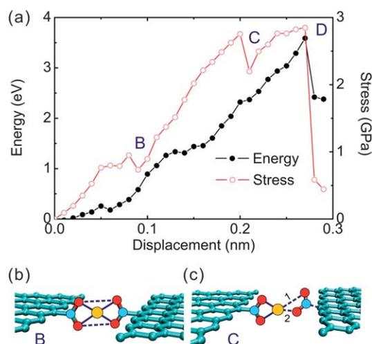
**Fig. 4** (a) Intralayer energy and stress profiles of carboxylate group inter-linked graphene sheets under tensile loading. When stretched, the Mg–O complex is firstly straightened and the magnesium atom is pulled back to the plane formed by the oxygen atoms (a) at “B”. The structure fails and the Mg–O bonds break in sequence (first bond “1” in (c) at “C”, then bond “2” at “D”). The tension displacements in (b) and (c) are labeled in (a) with B and C.
