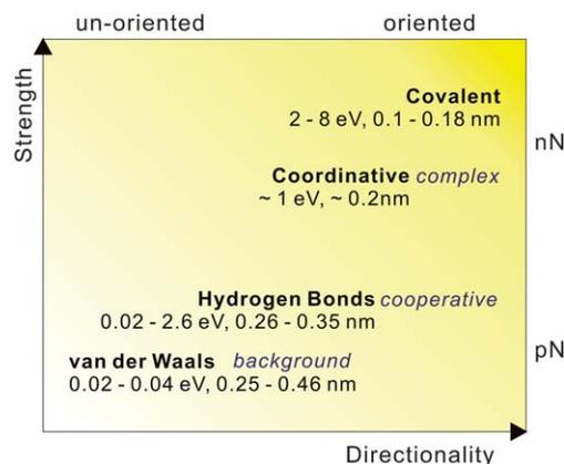
**Fig. 5** Comparison of different crosslink mechanisms in graphene nanocomposites, in terms of strength and directionality. The typical energy value and bond length are also given in the units of eV and nm. The binding energy of hydrogen bonds covers both weak and strong hydrogen bonds as classified in ref. 21, the bond length is the distance between the electron donor and acceptor.
