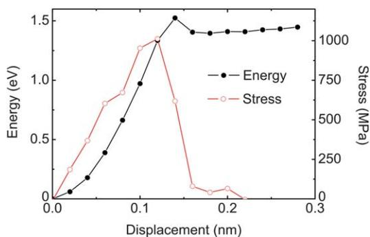
**Fig. 3** Energy and tensile stress profile of coordinative bonds bridging graphene bilayers (structure I) under tensile load in the normal direction to graphene sheets.
