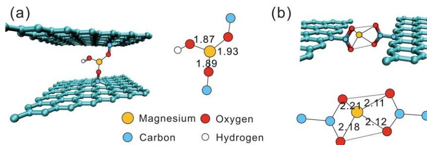
**Fig. 1** Structures of divalent ion based crosslinks that bridge graphene sheets. (a) Is an interlayer crosslinker as reported in ref. 10. The bond lengths in the local structures are depicted in Å. (b) Is the intralayer crosslinker that provides a coordinative connection between oxygen atoms in neighboring graphene sheets and the magnesium atom buckles out of the plane. These two structures show Mg–O bond lengths between 0.19 to 0.21 nm.
