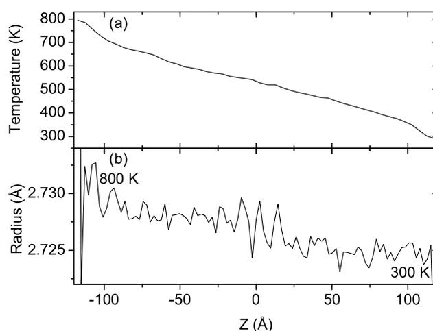
**Figure 4.** Variation of the (a) temperature and (b) local radius of the inner tube along its length. The hot and cold ends (left and right, respectively) are maintained at 800 and 300 K, respectively.
