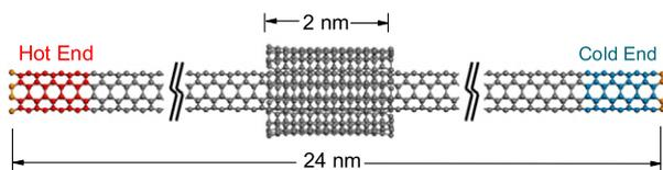
**Figure 1.** Schematic of the (4, 4)/(9, 9) model DWNT used to study thermally driven motion. Edge atoms at both ends (in orange colour) are fixed in position, while red and blue coloured regions are thermostated at relatively high and low temperatures, respectively.
