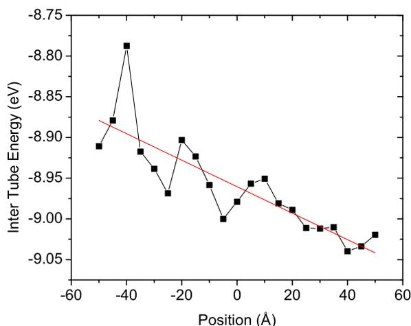
**Figure 5.** Variation of inter-tube van der Waals energy with different initial positions of the outer tube in the (4, 4)/(9, 9) DWNT configuration. The hot and cold ends of the inner tube are maintained at 800 K and 300 K, respectively.
