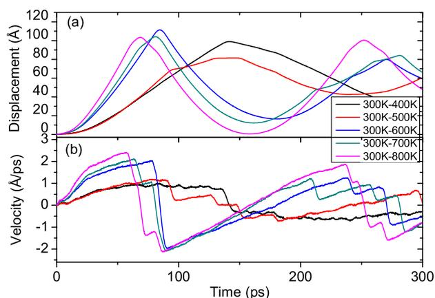
**Figure 2.** (a) Displacement and (b) velocity of the centre of mass of the outer (9, 9) tube as a result of different thermal gradients applied across the inner (4, 4) nanotube.
