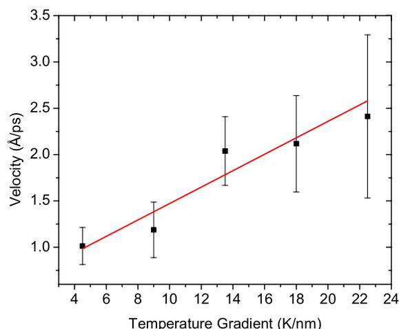
**Figure 3.** Averaged terminal velocity of the outer tube as a function of different thermal gradients of 4.5, 9, 13.5, 18 and 22.5  $\text{K nm}^{-1}$ .
