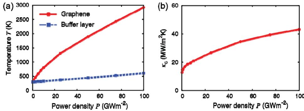
**Figure 3.** Power density dependent interfacial thermal conductivity. (a) The temperature evolution in the graphene sheets at various power density  $P$  from 0.1 to 100  $\text{GW m}^{-2}$ . (b) Interfacial thermal conductivity between graphene and 6H-SiC substrate as calculated from  $\kappa_c = J/(\Delta TA)$ , where  $\Delta T$  is the temperature difference across the interface with area  $A$ .
