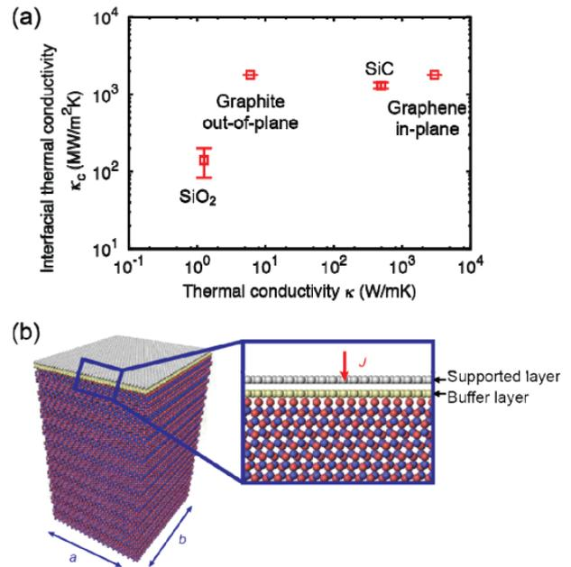
**Figure 1.** Thermal transport across interfaces with graphitic structures. (a) Thermal conductivity  $\kappa$  and interfacial thermal conductivity  $\kappa_c$  of several representative materials and their interfaces with graphene or carbon nanotubes [33–36]. (b) A schematic illustration and the atomic structure of graphene–6H-SiC interface.
