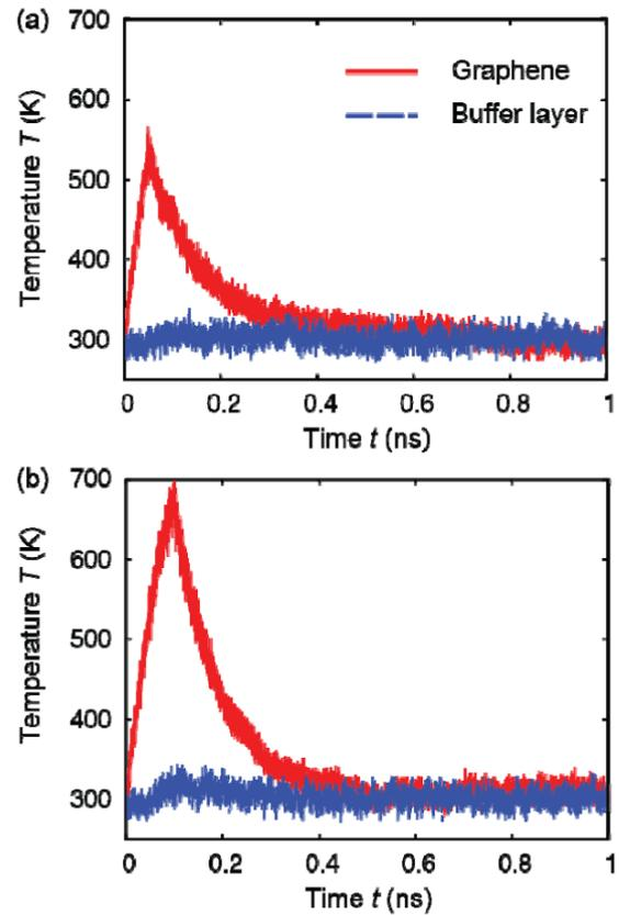
**Figure 4.** Temperature evolution profiles in the graphene sheet and buffer layer after short heat pulses  $P = 10 \text{ GW m}^{-2}$  are generated for (a) 50 ps and (b) 100 ps. The exponential decay of temperature in the graphene sheet is fitted to calculate the interfacial thermal conductivity.
