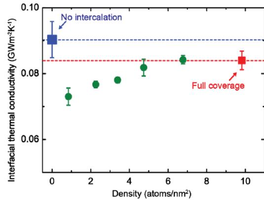
**Figure 6.** Interfacial thermal conductivity  $\kappa_c$  calculated for graphene layers intercalated with argon atoms, as a function of its areal density.  $\kappa_c$  without intercalation. The results for the case of full monolayer coverage are also plotted for reference.
