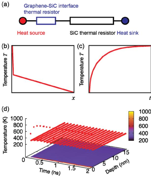
**Figure 5.** (a) Schematic illustration the two-resistor model. (b) and (c) The temperature profile  $T(x)$  evolution  $T_G(t)$  in the graphene sheet and 6H-SiC as predicted by using the Fourier’s diffusive model for heat transfer. (d) The distribution and time evolution of temperature  $T(x, t)$  in the hybrid graphene–SiC system at  $P = 10 \text{ GW m}^{-2}$ , as a function of time  $t$  and depth  $x$  from the supported graphene into the substrate.
