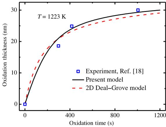
**Fig. 2.** Comparison of the model predictions and experimental results of the oxidation of a Si NW with radius  $R = 25$  nm. Symbols denote experimental results, and solid and dash lines refer to the predictions by the present and 2D Deal-Grove model, respectively.
