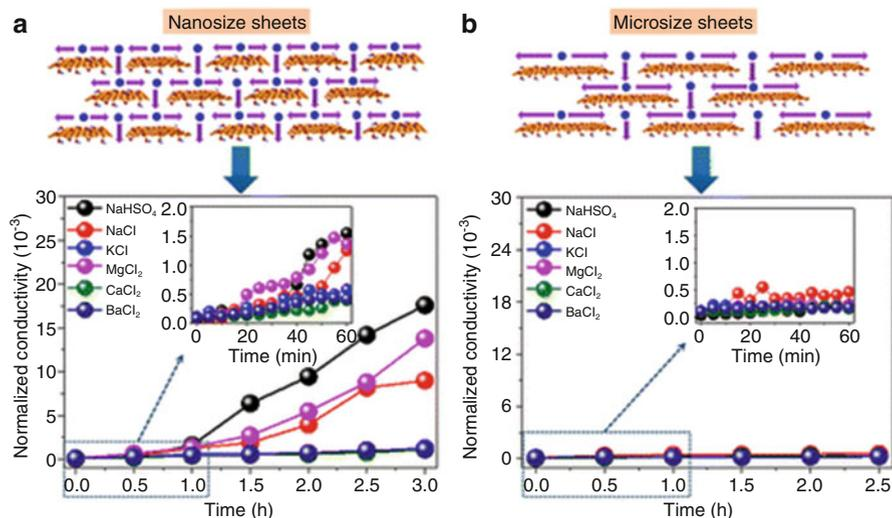
**Fig. 5.7** Schematics of the lamellar structures and conductivities of cations across GO membranes composed of (a) nanosized and (b) micro-sized GO sheets. *Insets* show the initial stage (0–60 min) measurements of the penetrations [18–20]. (Reproduced by permission from ACS)
