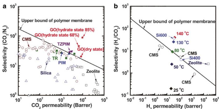
**Fig. 5.8** (a) Relation between  $\text{CO}_2$  permeability and  $\text{CO}_2/\text{N}_2$  selectivity of GO membranes under dry and humidified conditions. (b) Comparison of gas separation performance between GO membranes and other membranes for the  $\text{H}_2$  permeability and  $\text{H}_2/\text{CO}_2$  selectivity [16]. (Reproduced by permission from AAAS)
