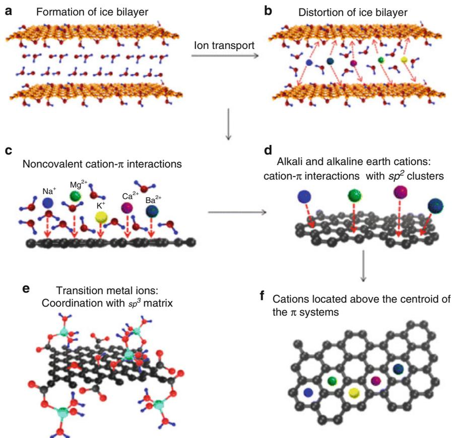
**Fig. 5.5** Schematic diagrams of selective ion transport through GO membranes and the diverse interactions between different cations and GO [18–20]. (Reproduced by permission from ACS)
